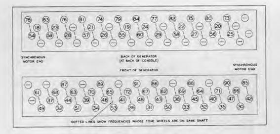
Figure 1-3. Magnet Location on Tone Generator
