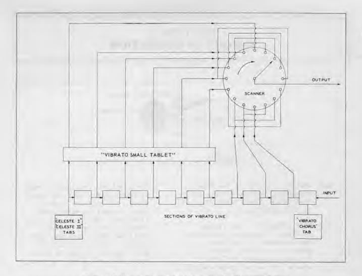
Figure 2-2. Fundamental Diagram of Vibrato System
