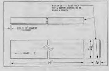
Figure 4-1 Bottom Rail Construction
